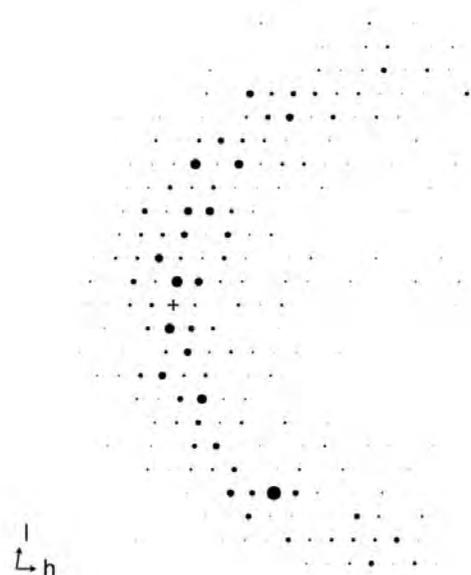
**Figure 6** One diffraction pattern from the series of patterns that were summed in the precession multislice code for GITO at an azimuthal angle of  $\pi/2$  and a cone semi-angle of 24 mrad. A close to systematic row condition is excited along the  $I$  direction for this tilt. The diffraction spot areas are proportional to intensity
